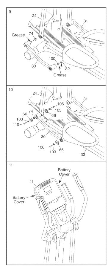
12. **Make sure that all parts of the elliptical exerciser are properly tightened.** Note: Some hardware may be left over after assembly is completed. To protect the floor or carpet from damage, place a mat under the elliptical exerciser.
